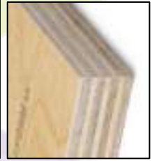
PLYWOOD STRUCTURE (odd number of thin layers of wood, glued together)
